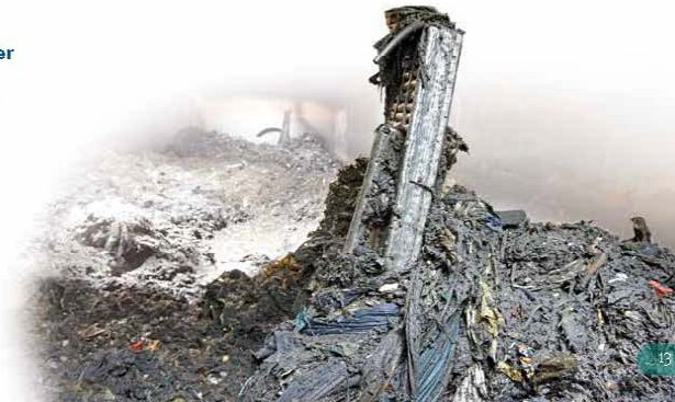
View of the agitator arm in the aggregate for the new DAMP® process: microbially-convertible organic materials remain in the solid material, thus optimising the next step of biological drying.
